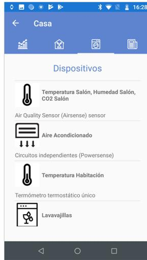
**Fig. 4.** Devices deployed within an Irish pilot house shown in the RESPOND mobile app.
